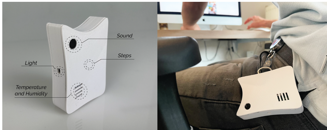
Figure 1: SensorBadge: Sensor implementation and in context when attached to the belt clip
